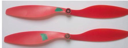
FIGURE 3.6 – Hélices 10"4.5" calibré
