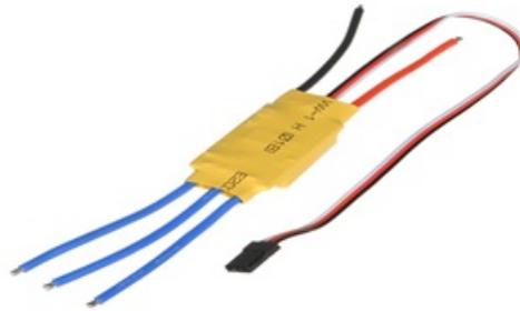
FIGURE 3.5 – Electronic Speed Control
