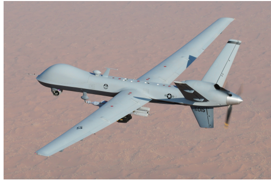
Figure 1.4: The General Atomics MQ-9 Reaper (Predator B) is a High Altitude Long Endurance UAV
