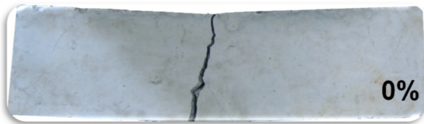
Figure II.2 : Fissuration en Béton sans fibres [2]
