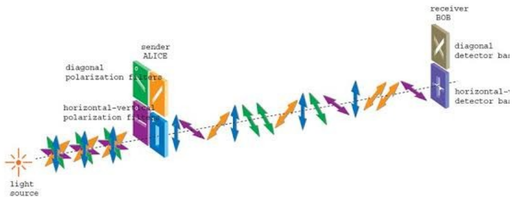
Figure II.10 : Principe de protocole BB84.
