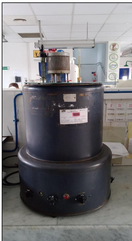
Figure III.5 : Appareillage de la TVR ASTM D323
