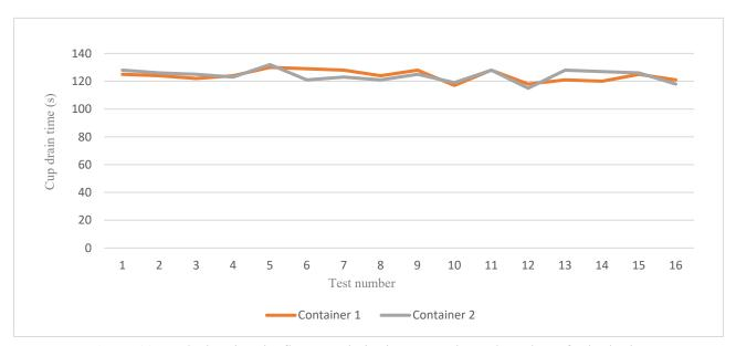
Figure 30 graph showing the flow cup drain time on each conducted test for both glue containers.
