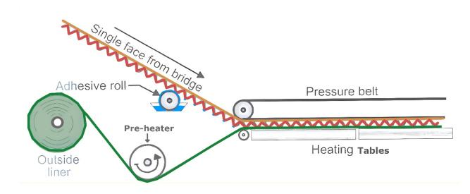
Figure 21 Simple diagram of the double facer in the wet section of the corrugation machine.
