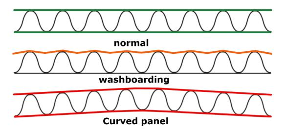
Figure 28 Different phenomenon's that can occur during production of cardboard panels.
