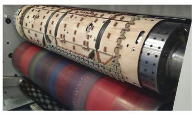
Figure 25 Rotary cutting mold.
