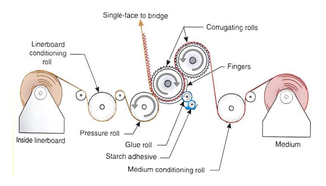
Figure 20 Simple diagram of the single facer in the wet section of the corrugation machine.
