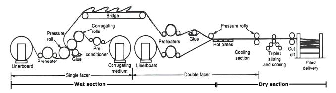
Figure 19 Simple diagram of a corrugation machine.
