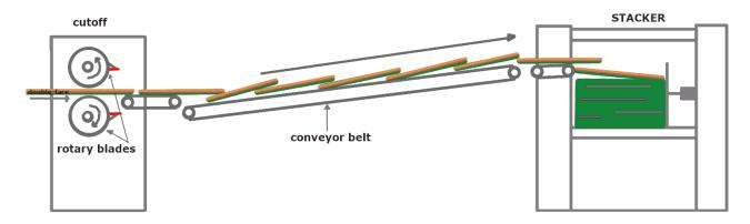
Figure 22 Simple diagram of the dry section of the corrugation machine.
