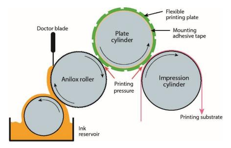
Figure 26 Simplified diagram of the printing process using flexography
