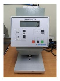
Figure 15 Image of a L&W Micrometer.
