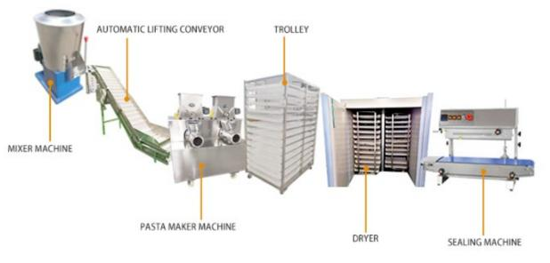
Figure 2 Image of a pasta production line layout (automaticfoodprocessingmachines.com)
