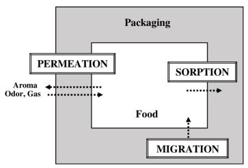
Figure 5 Diagram showing container-content interactions
