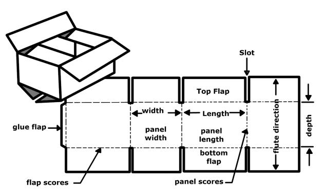
Figure 13 Regular Slotted Container (RSC) design layout
