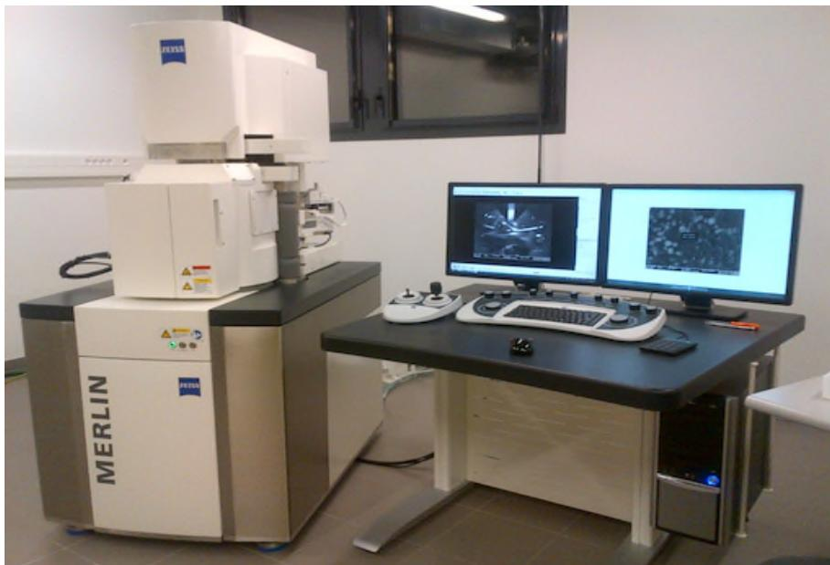
**Figure II-11 :** Appareil MEB.
