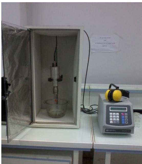
**Figure n° 6:** Ultrasound assisted extraction system.
