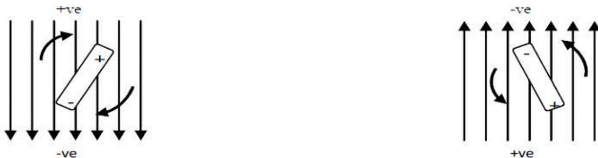
Figure n° 2: Movement of a dipole in an electric field (Singh and Heldman, 2001).
