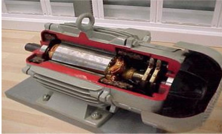
**Figure (I.21):** Machine synchrone [24]
