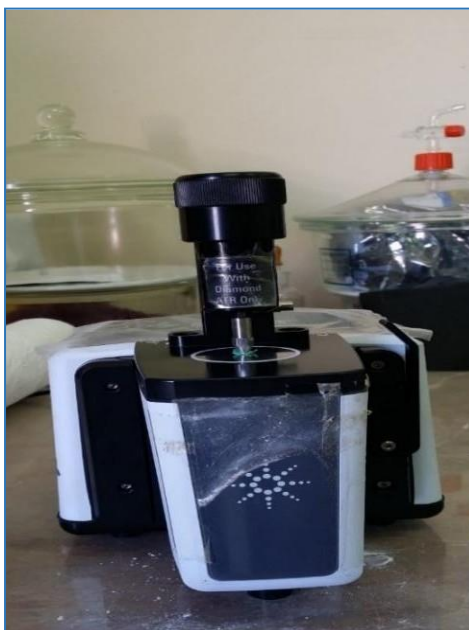
Figure III.8: Spectrophotomètre type Agilent Technologies Cary 630 FTIR (ATR)
