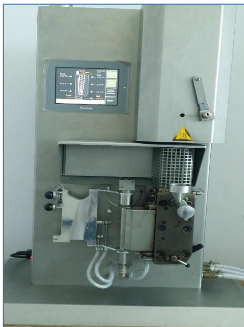
Figure III.2: l'extrudeuse DSM Xplore Netherlands.
