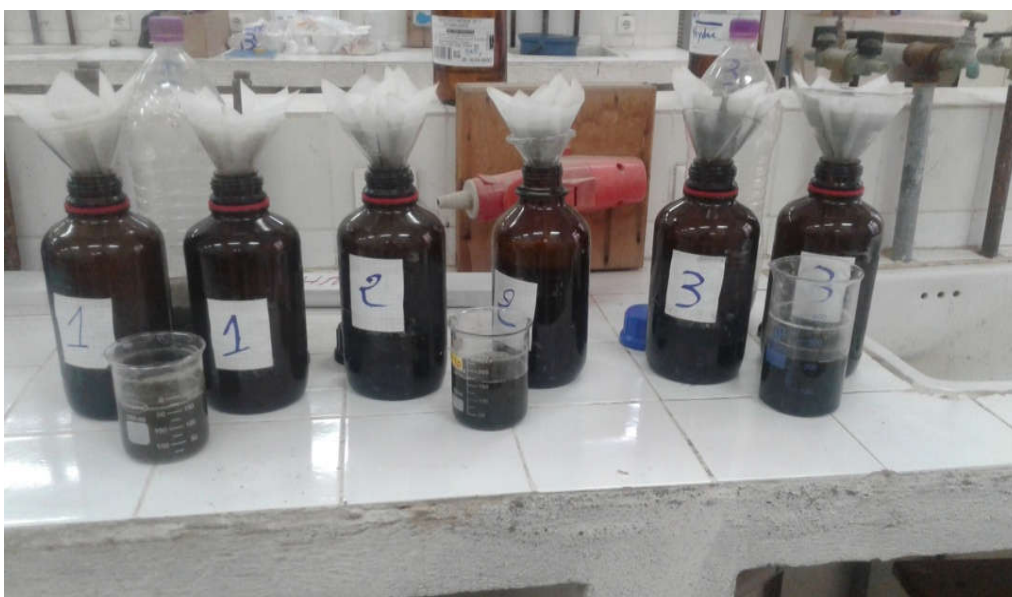
Figure II.3. Filtration du lixiviat
