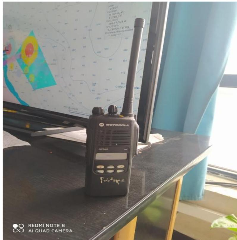
**Figure II.2 :** VHF portable.
