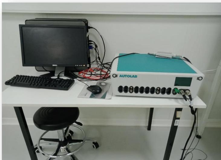
Figure III.5 : Potentiostat/Galvanostat PGSTAT302N.
