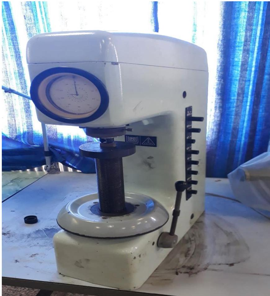
Figure III.7: Durometre HRC.
