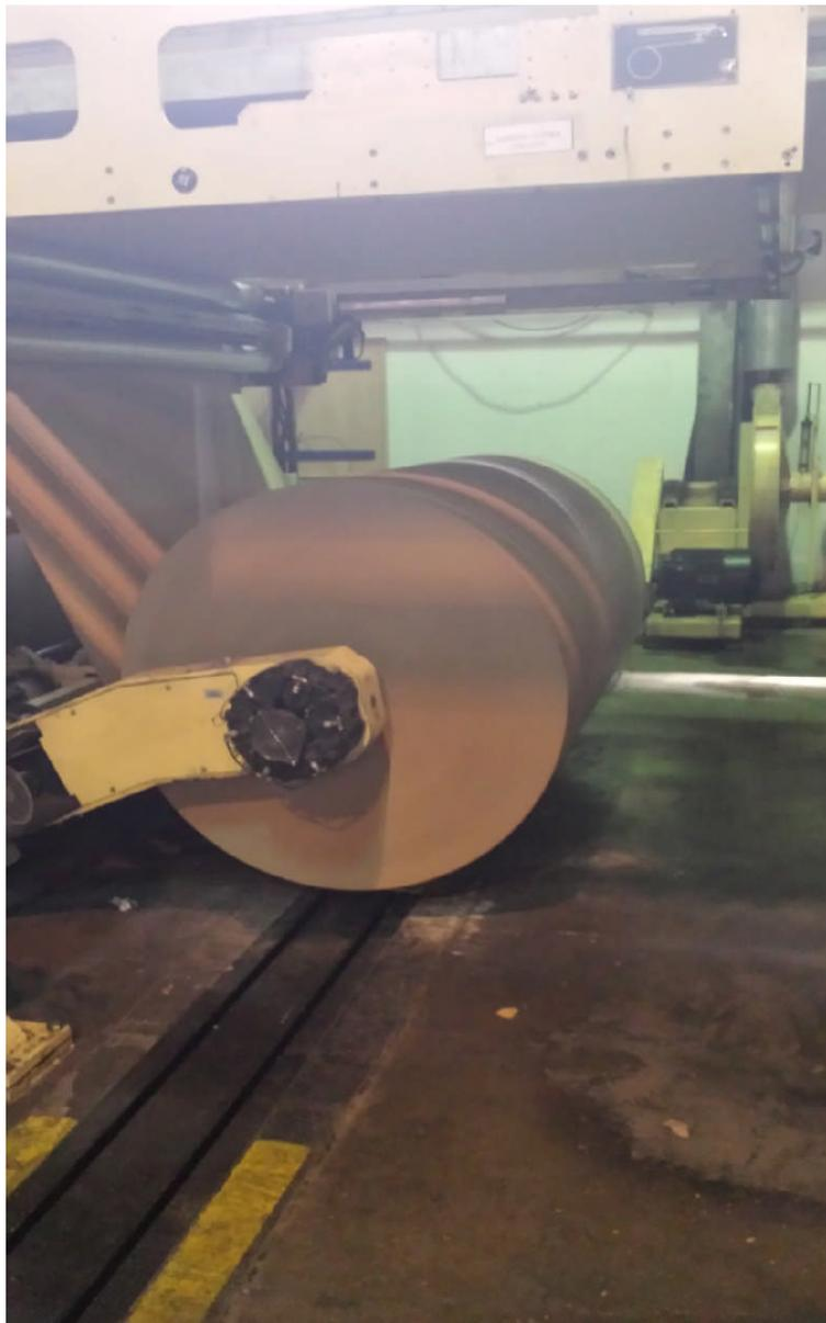
**Figure II. 7: la simple face type COM VFL [1]**
