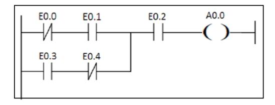
Figure V-2 Exemple de langage ladder (LD)
