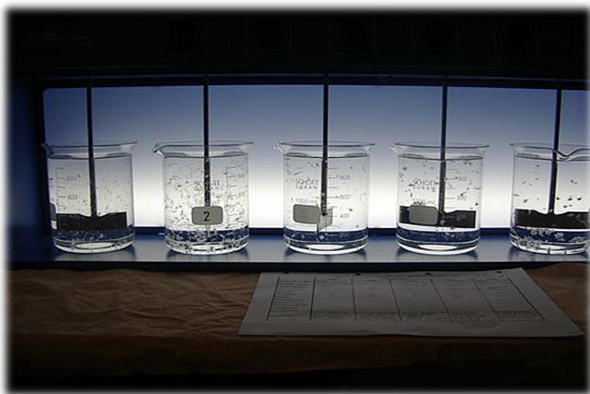
**Figure 9-** Coagulation-floculation (jar-test).
