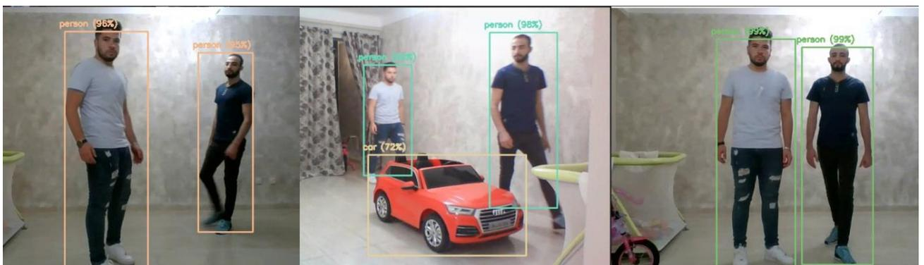
Figure IV.19: Examples of detected frames on Raspberry-Pi Client while using person-vehicule model
