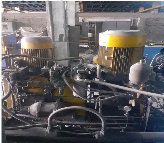
**Figure II.12 :** Centrale hydraulique (Hydraulikplan HA NG 250)
