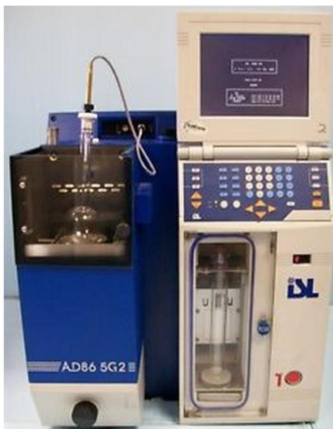
**Fig.V.2** : Appareil de distillation ASTM D86
