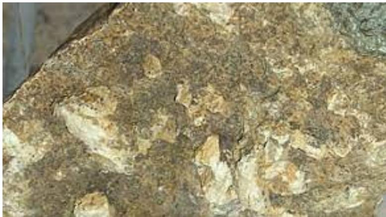
**Figure III.4 :**hydroxyapatite naturelle  $\text{Ca}_5(\text{PO}_4)_3(\text{OH})$
