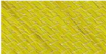
**Figure .I.7.** fibre d'aramide [21]
