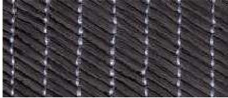
**Figure .I.6.** fibre de carbone [19]
