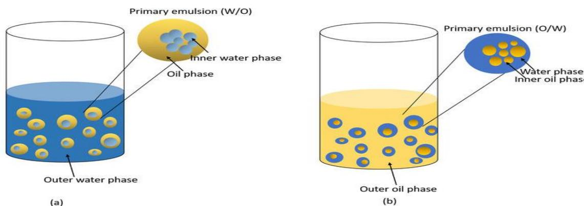
**Figure 03:** Schema of a) W/O/W and b) O/W/O emulsions (Fraj et al., 2021).
