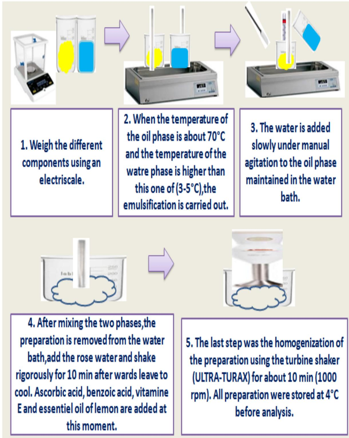
**Figure 08:** Schematic of the preparation of cosmetic creams (Hua et al., 2019; Moldovan et al., 2021).
