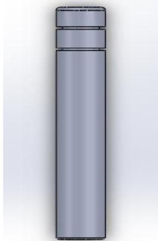
FIGURE II 30: COLONNE DE GUIDAGE.
