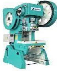
FIGURE II 1: PRESSE MECANIQUE
