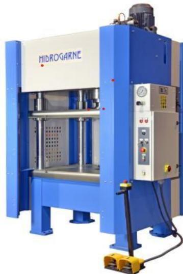
FIGURE II 8: PRESSES A COLONNES.
