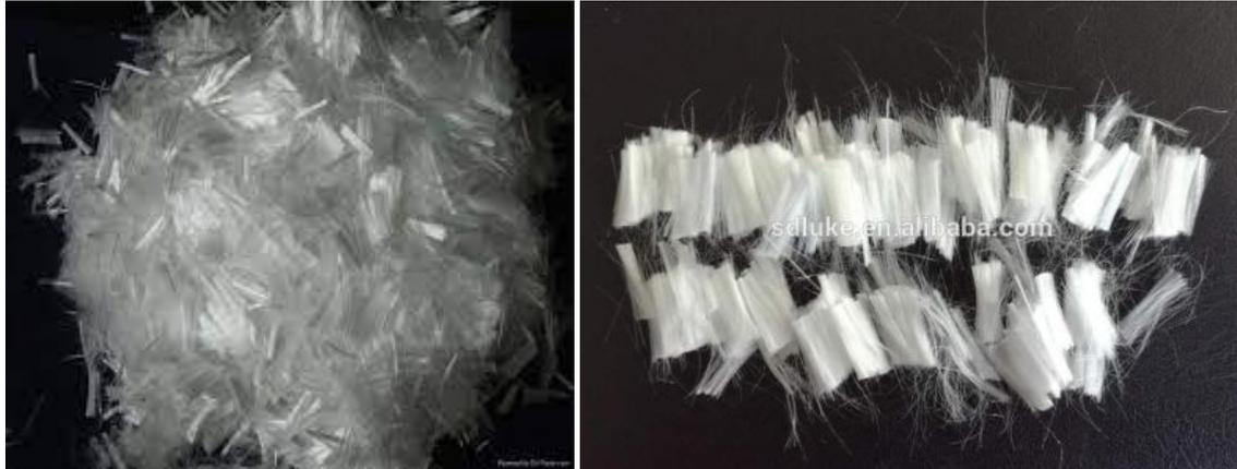
**Figure I.21:** fibre polypropylène
