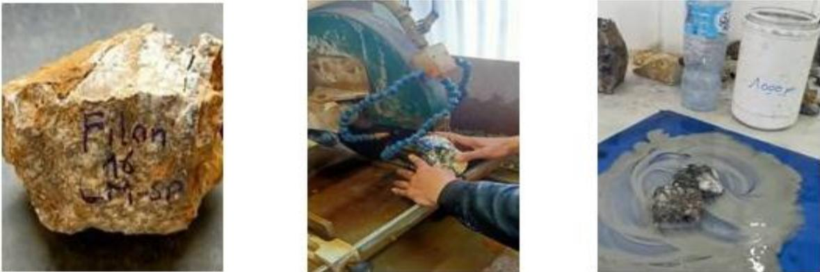
Figure III.40. Echantillon + sciage + rodage [photos prises]
