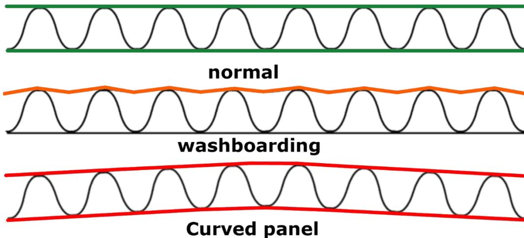
Figure 28 Different phenomenon's that can occur during production of cardboard panels.
