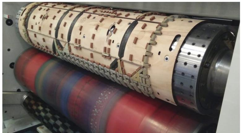
**Figure 25** Rotary cutting mold.
