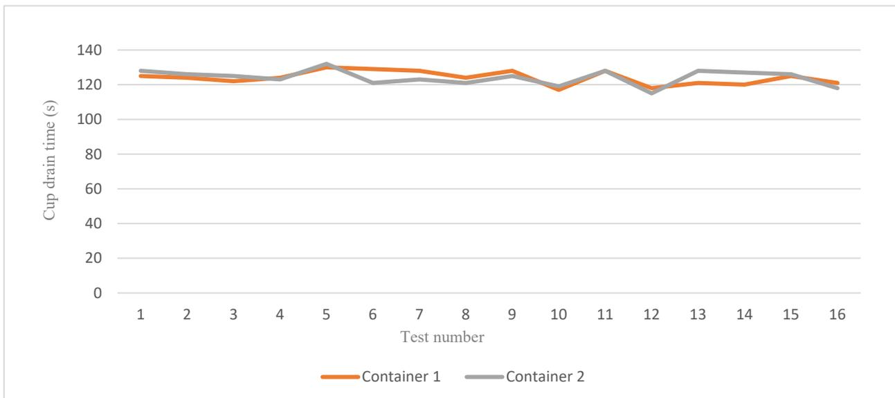
**Figure 30** graph showing the flow cup drain time on each conducted test for both glue containers.
