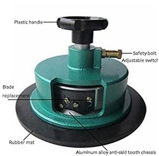
**Figure 17** Image of a Circular Cutting knife
