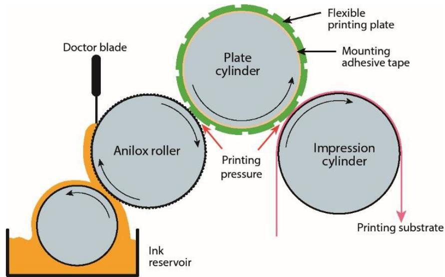
Figure 26 Simplified diagram of the printing process using flexography
