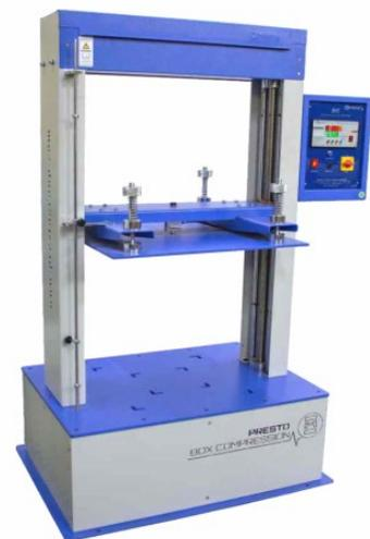
**Figure 16** Image of a BCT testing machine.
