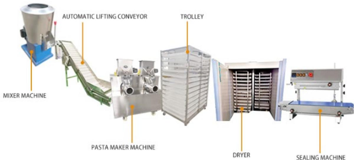
**Figure 2** Image of a pasta production line layout
