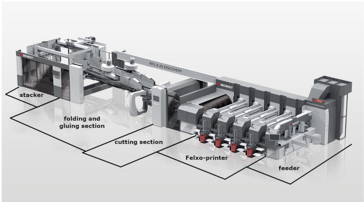
Figure 23 BOBST 820 and its transformation sections
