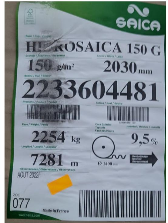
Figure 12 Technical specification sheet of HidroSaica 150 G paper.
