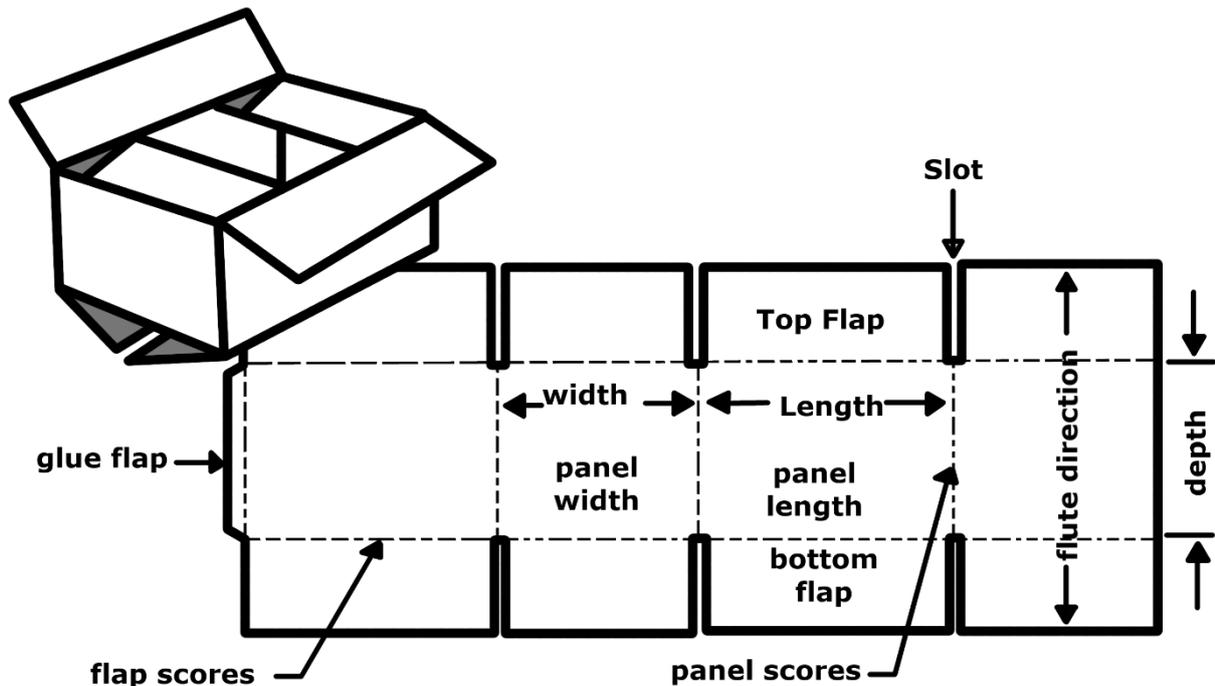
Figure 13 Regular Slotted Container (RSC) design layout
