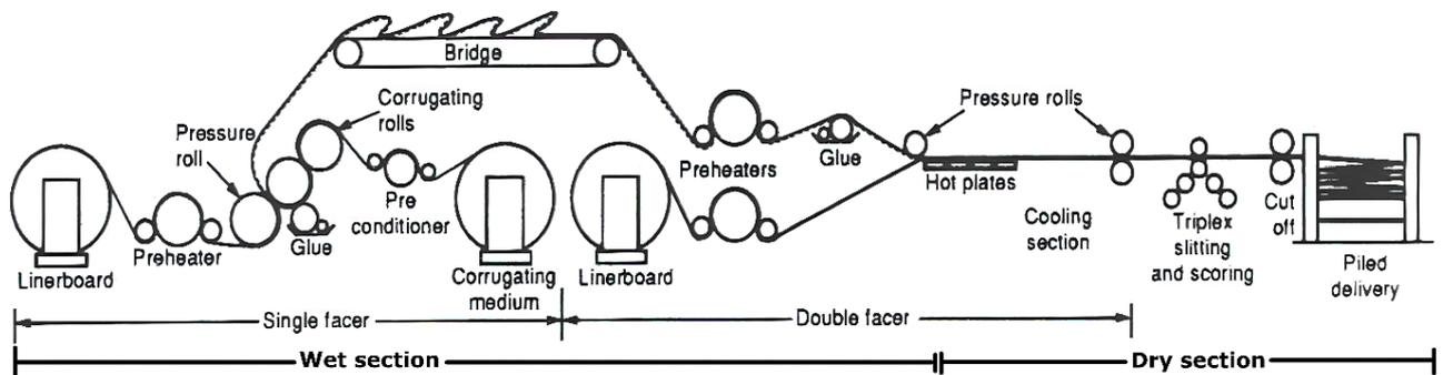
Figure 19 Simple diagram of a corrugation machine.
