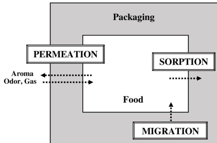
Figure 5 Diagram showing container-content interactions
