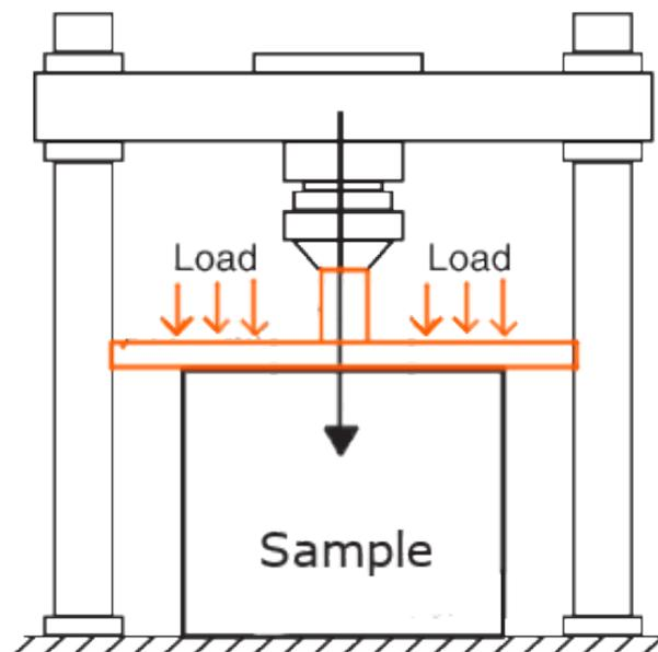
Figure 29 Simple diagram of the BCT test
