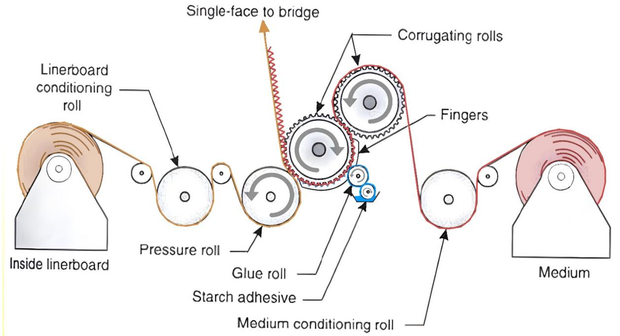
**Figure 20** Simple diagram of the single facer in the wet section of the corrugation machine.
