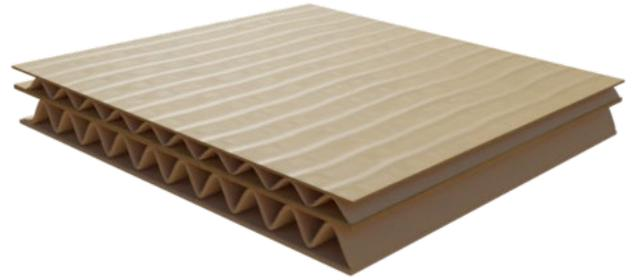
**Figure 7** Double-double-face corrugated cardboard panel.
