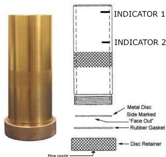
Figure 27 Stein Hall Viscosity cup and its diagram
