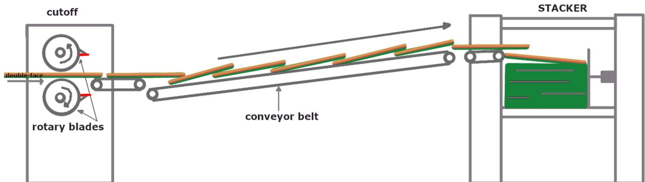
Figure 22 Simple diagram of the dry section of the corrugation machine.
