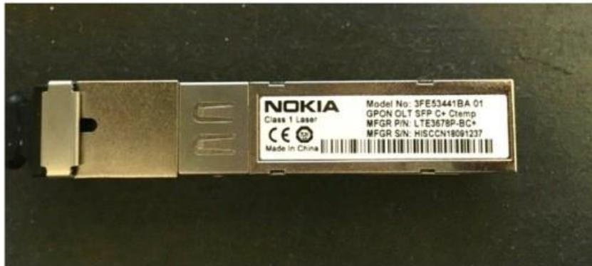
Figure II.6 : Module SFP GPON C+ [35].
