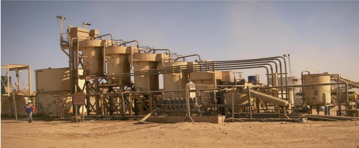
**Figure I-14 :** Colonnes de Charbon (photo prise).
