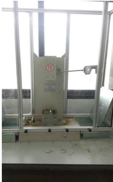
Figure II.15 : Appareil de choc (type Izod) JINAN TESTING
