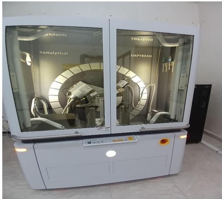
**Figure II.2.** Diffractomètre Malvern PANalytical Empyrian Series 3 X-ray.
