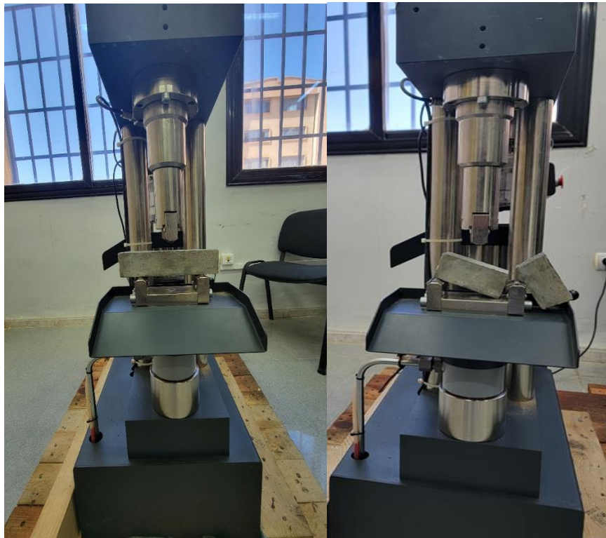
Figure II.24. Essai de la flexion trois-points.
