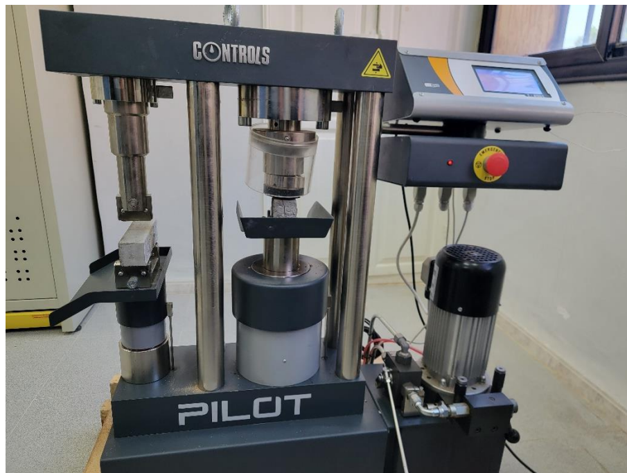
Figure. II.23. Machine de flexion ou de compression CONTROLS.
