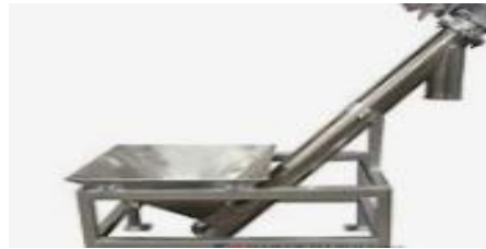
Figure 3:6 screw feeder mounted with hopper
