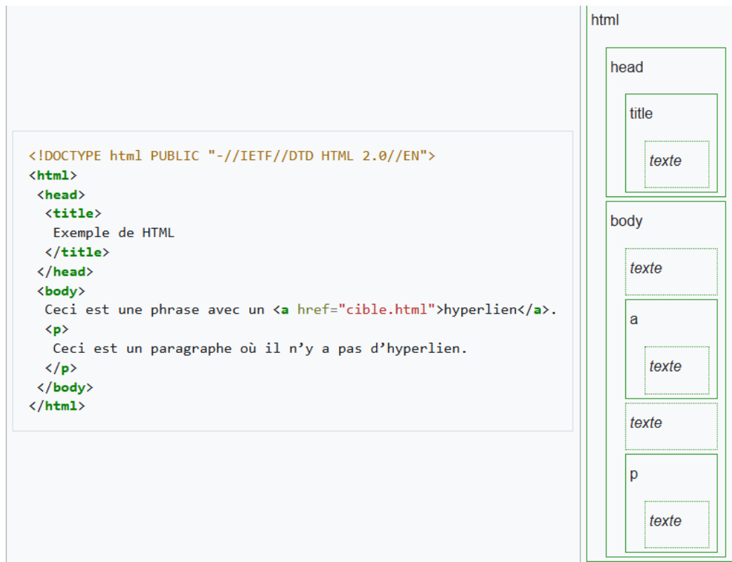
Fig. 3.2 : Structure of an HTML document
