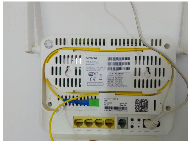
Figure 2.22: Optical network terminal rear view.
