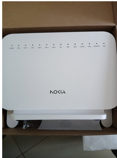
Figure 2.21: Optical network terminal front view.
