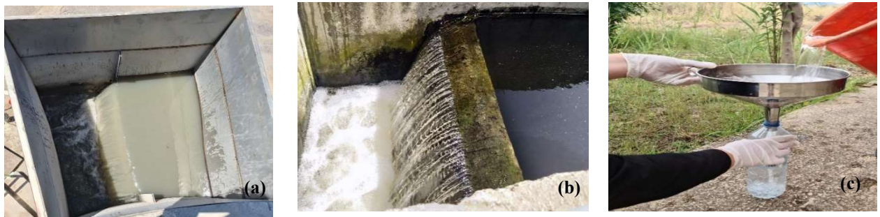
Figure 18. Sampling operation in the inlet and outlet of the wastewater treatment plant.
