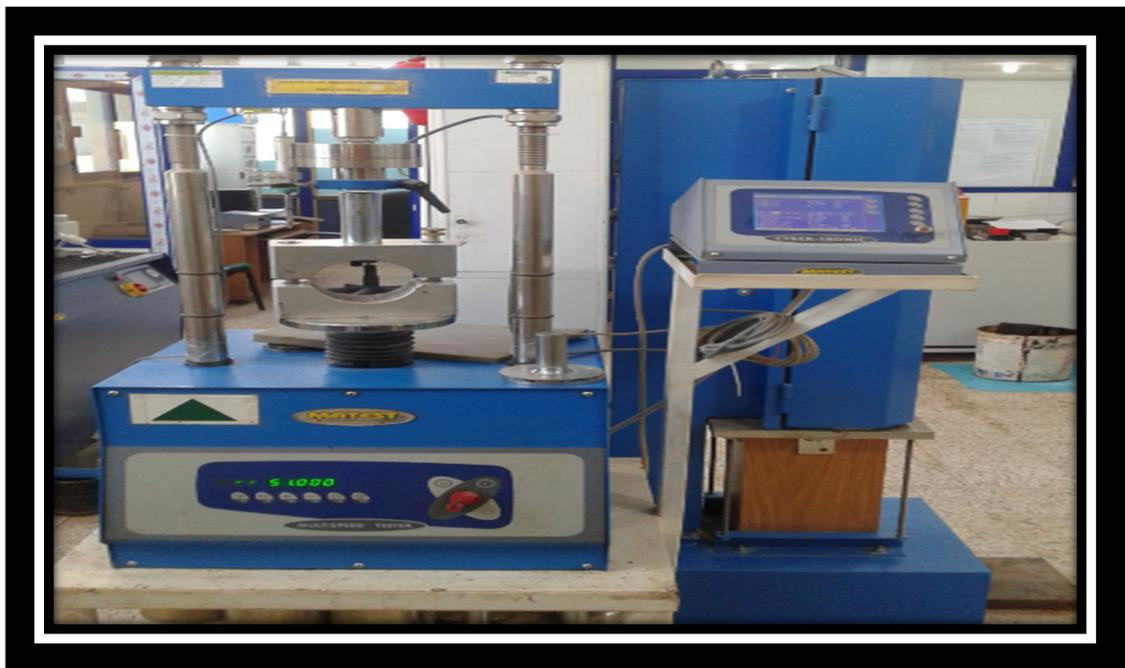
**Figure II.10 :** Appareille MARSHALL.
