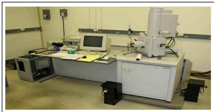
**Figure III. 5 :** Appareil MEB.
