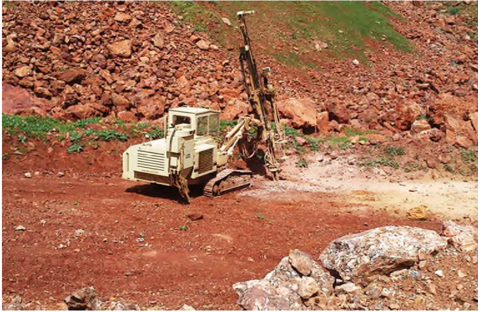
Figure III.1 : Foreuse ATLAS COPCO CM470.
