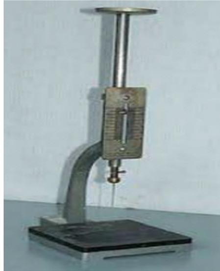
**Figure II.6.**Appareil de Vicat.
