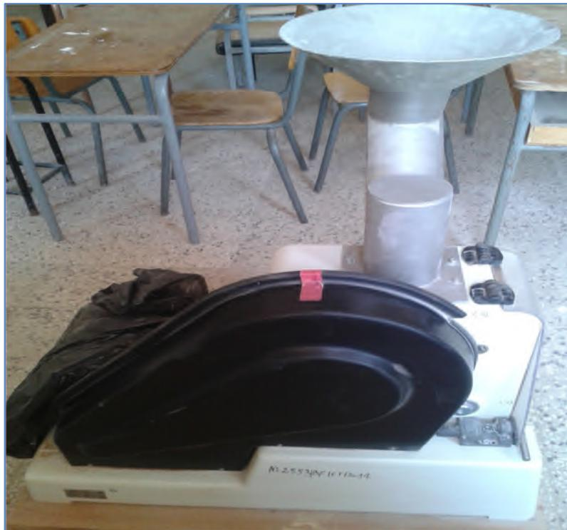
**Figure III.1:** Photo of our laboratory jaw crusher
