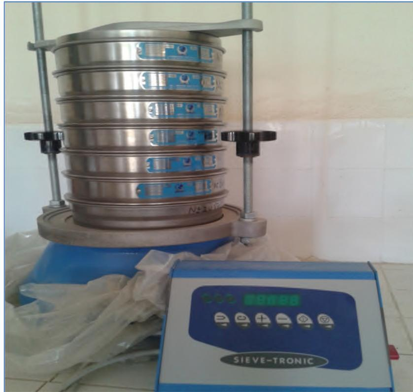
**Figure III.3:** Sieves column and its shaker
