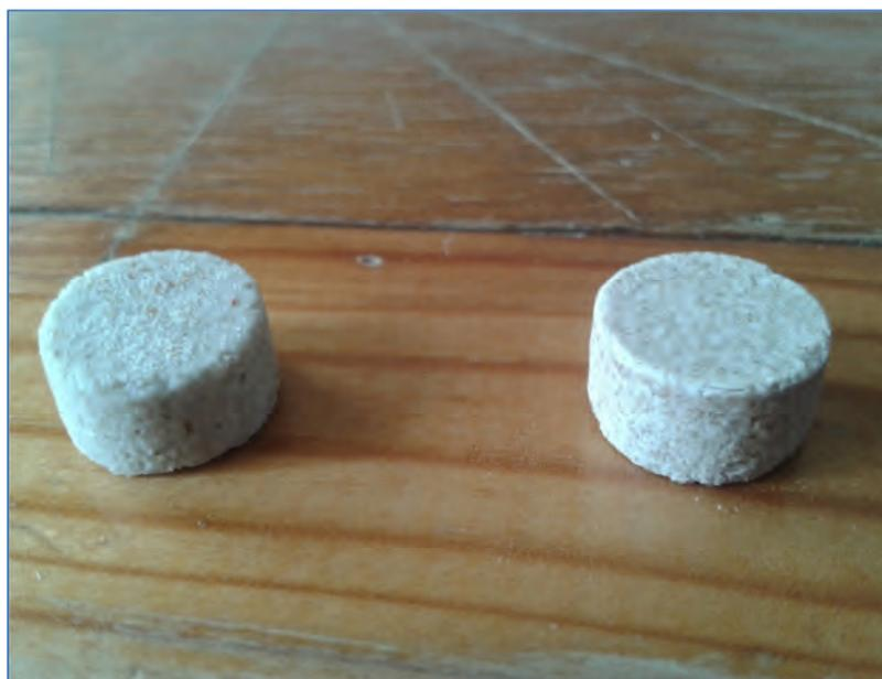
**Figure III.14:** Ceramics of 10% of barite after sintering
