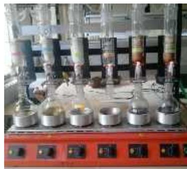
**Photo IV :** Appareil Soxhlet
