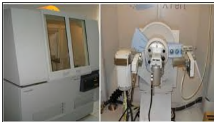
Figure 17: la machine de DRX expert prof panalytical.
