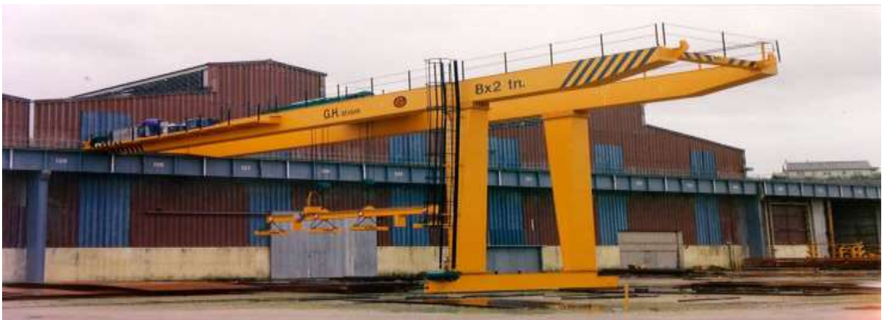
Figure I.8: Semi portique bipoutre.
