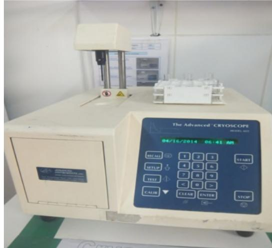
**Figure 03 :** cryoscope (model 4D3).
