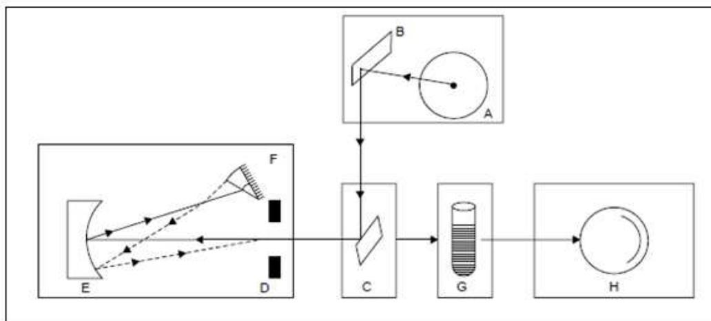
Figure 7 : Schematic representation of the optical system in a single beam spectrophotometer
