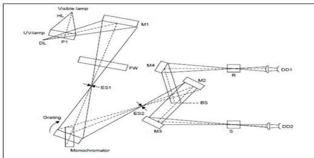
**Figure 8 : Schematic representation of the optical system in a double-beam spectrophotometer**
