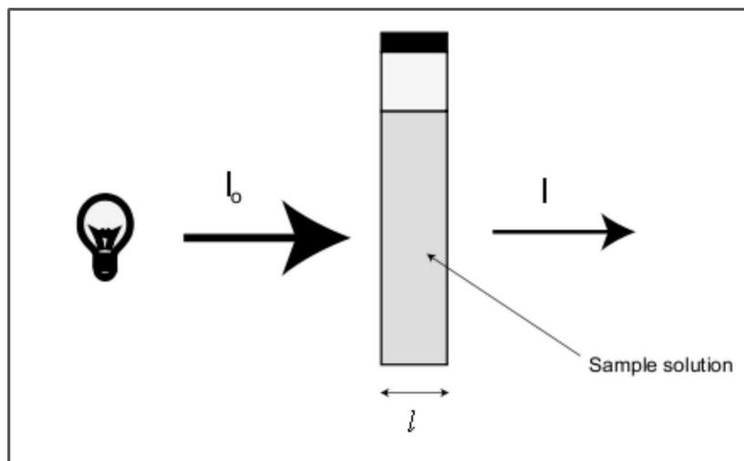
Figure 6 : Scheme of the principle of the beer's law .
