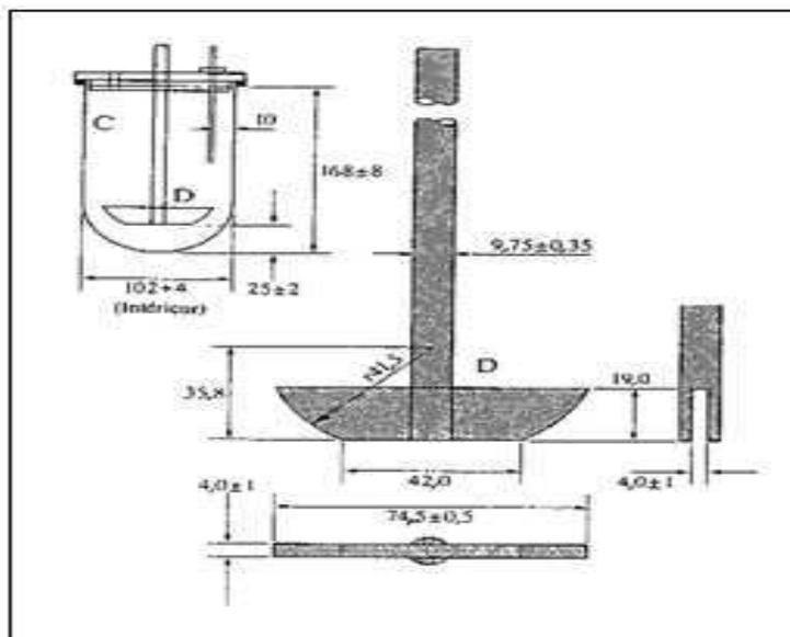
Figure 10 : Paddle Apparatus
