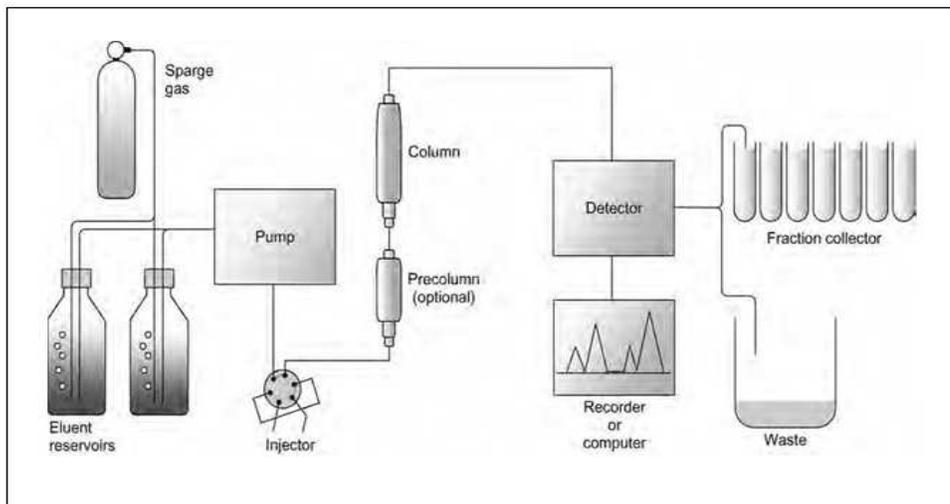
Figure 4 : A Typical HPLC System
