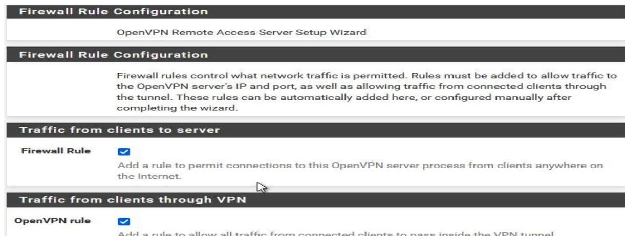
The screenshot shows the "Firewall Rule Configuration" page for the "OpenVPN Remote Access Server Setup Wizard".
