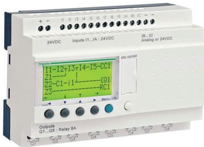
Figure II.5 : Automate programmable de type compact.
