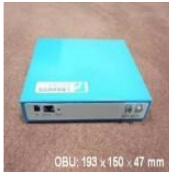
Figure 1.6 – Le dispositif OBU (On Board Unit) [13].
