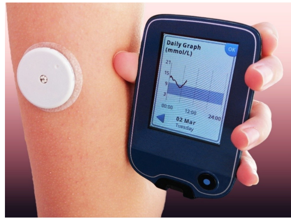
FIGURE 1.5 – Continuous Glucose Monitoring (CGM) (MEDICAL n.d.).
